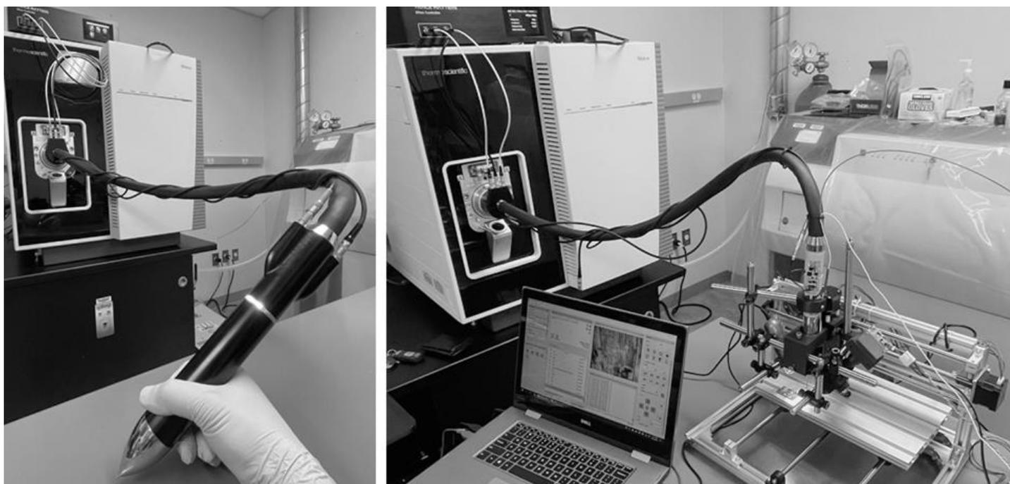
Figure 2. Examples in which SPion System™ is being used with a mass spectrometer: (left) SPion Inlet™ as a hand-held probe that can be moved around (ion source not included), and (right) a robotic stage implementation of SPion Inlet™ for imaging applications with laser/ESI ion source. The length of SPion Tube™ shown in these figures is 120cm (4 feet). SPion Tube™ can be made longer than pictured.
